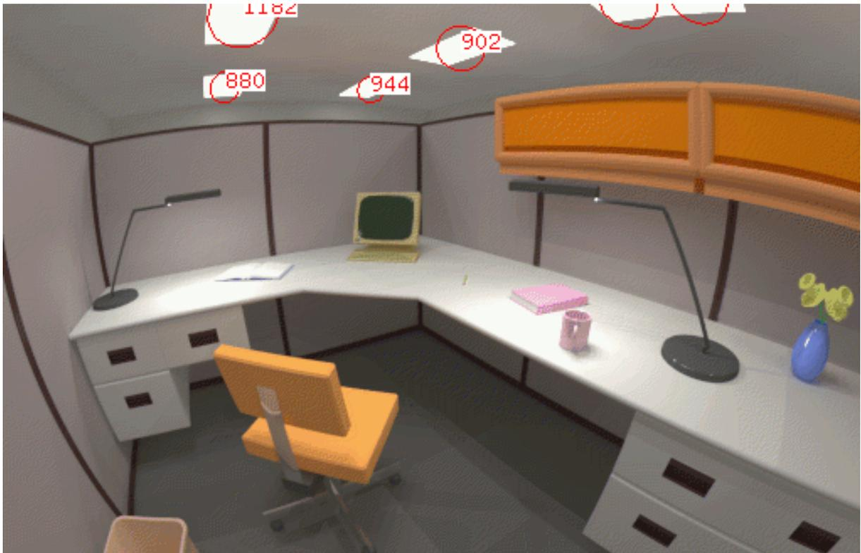
**Figure 8a.** Visual comfort probability (VCP, glare) calculation for cubicle office space, showing position and intensity of glare sources, computed with *Radiance*.
