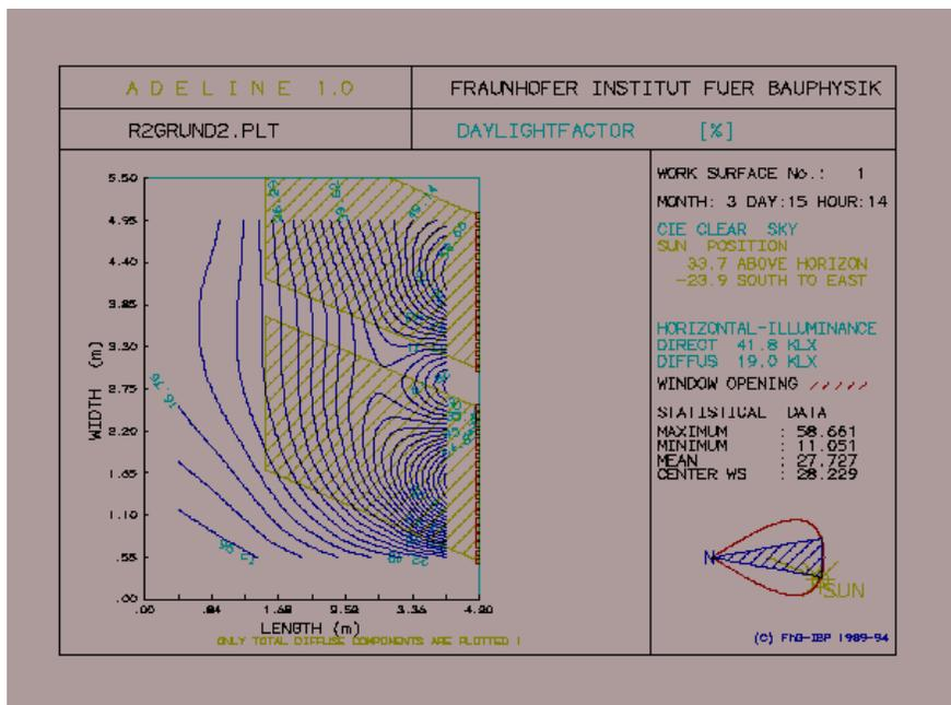
**Figure 7.** Daylight factor contours for workplane of two-windowed office space (empty), computed by *ADELIN*E. Sun patches are shown as yellow, hatched regions.
