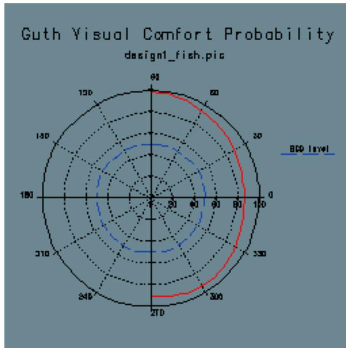
**Figure 8b.** Visual comfort probability (VCP, glare) calculation for cubicle office space, showing a numerical plot of VCP. The zero degree view is looking straight ahead in the image shown, and positive angles look to the right. A VCP of 75% means 75% of occupants are comfortable.
