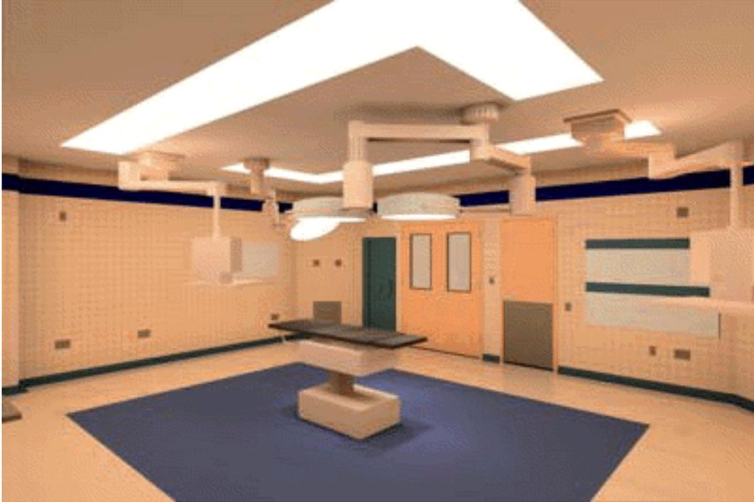
**Figure 11.** Radiosity solution of operating room, computed by *Lightscape*. Real-time movement through this scene is possible on a moderately-priced graphics workstation, without textures.
